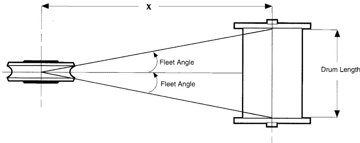
**X** = Minimum Distance from Drum to First Sheave or Load Connection – Feet
